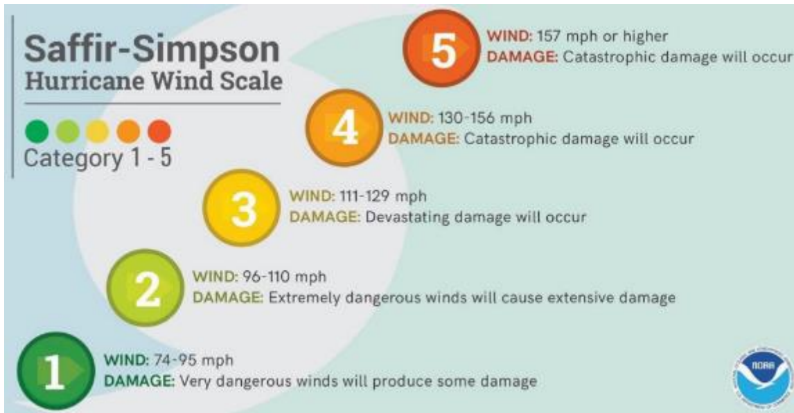
Figure 4.3.8-5. Saffir-Simpson Hurricane Wind Scale
